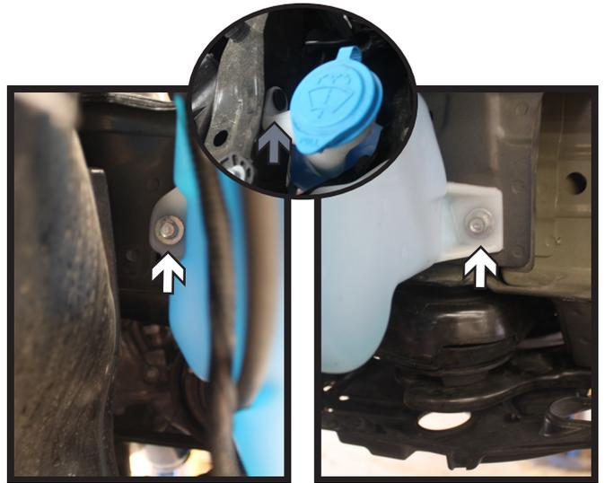
6. Using a 10MM socket, remove the two (2) screws from washer reservoir (white). Remove the push pin from the filler neck next to the cap (gray). Disconnect all lines from the reservoir and set aside.
