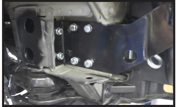
10. Continue to drill the remaining holes thru the frame. Install 3/8"-16 x 1-1/2" bolts with a 3/8" lock washers into the holes and secure with a 3/8" nut plates on the inside of the frame. Do this on both sides of the vehicle. Fully tighten all fasteners.
